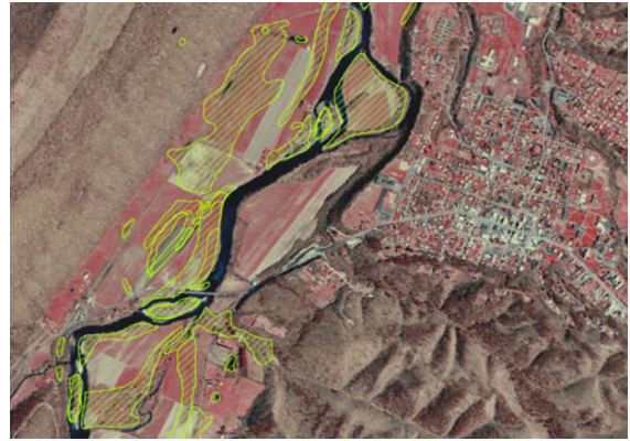
Fig. 6 The shaded areas represent potential wetland and stream mitigation banking sites for evaluation in Level 2 reconnaissance surveys. Shaded areas are a combination of SSURGO soils (NRCS 1995), National Wetland Inventory wetlands, and permeable land cover. This example is from the South Branch Potomac Watershed, West Virginia
