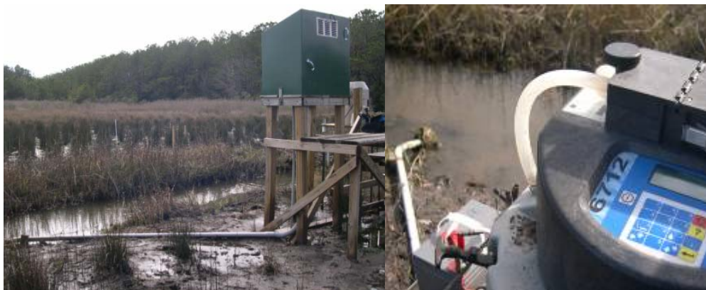
Figure 1. Example ISCO Sampler Setup
