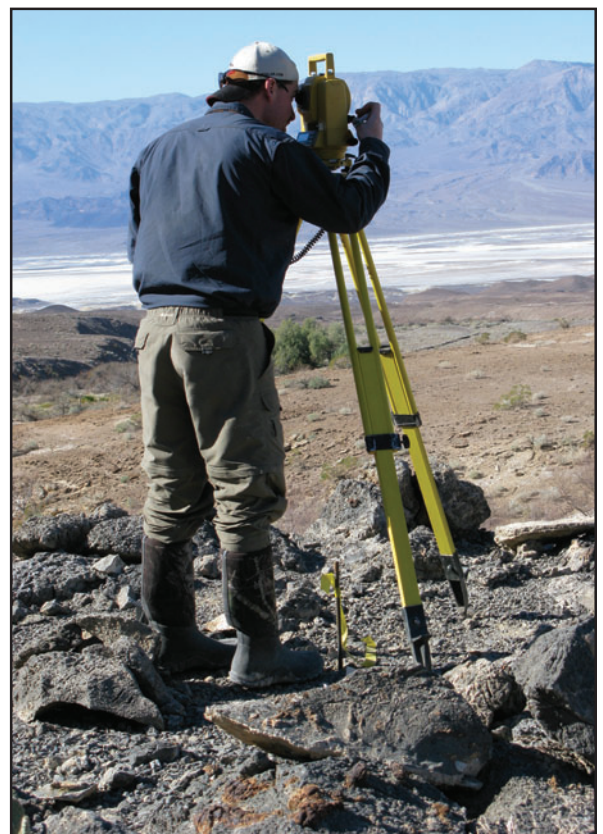
Figure 4-18. Topographic surveying with full station in Death Valley National Park, California.
