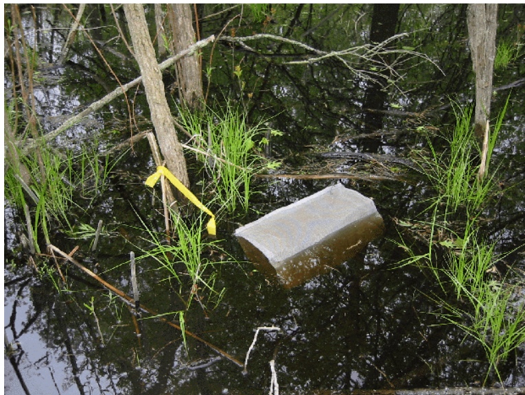
Figure 41. Funnel (activity) trap for amphibian and macroinvertebrate sampling. Aluminum window screening 28" x 18" is rolled into a cylinder 18" long and stapled through 1" lip to form a tube 8" in diameter. Fiberglass screening is cut out and stapled to form a funnel with an opening of 9" on the wide end and 1.75" on the narrow end. The narrow end of the funnel is placed inside the cylinder as indicated in the figure. The wide end of the funnel is rolled over the outside edge of the cylinder and stapled every 0.5". A string handle is attached to the lip. The trap is emptied by everting the fiberglass funnel at one end and dumping the contents into a white tray.
