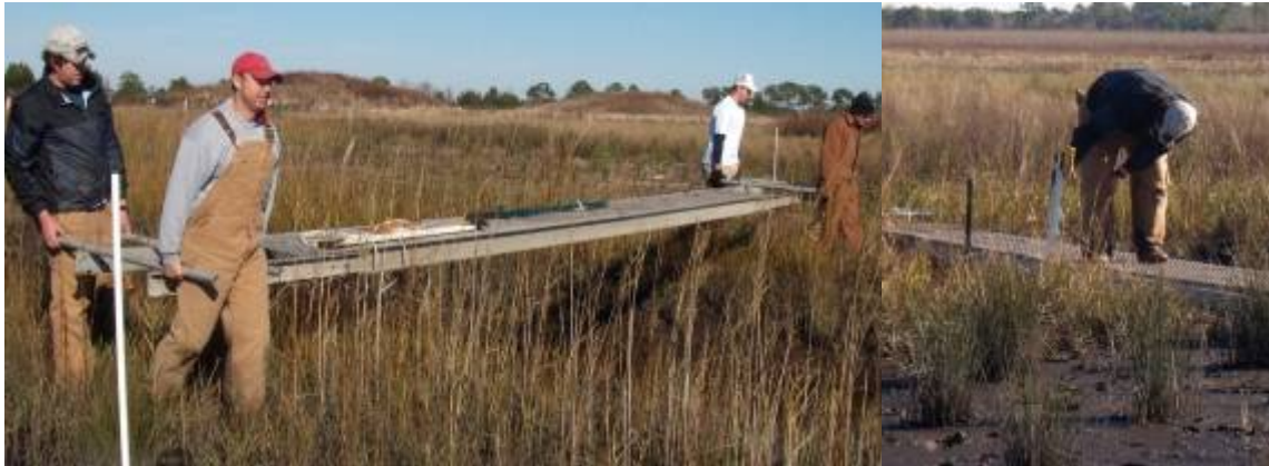
Figure 2. Sag tape surveying method
