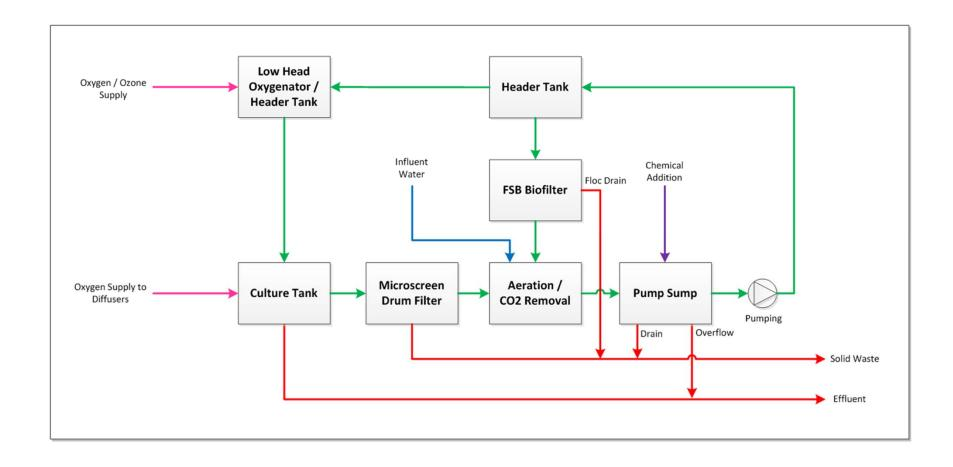
Two process loops through a centralized, forced-air CO2 stripper
