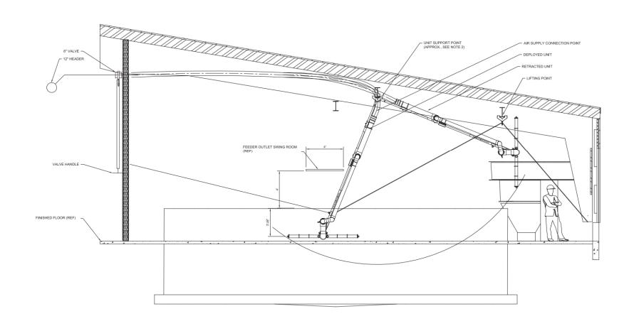
**Device is suspended and retractable**
