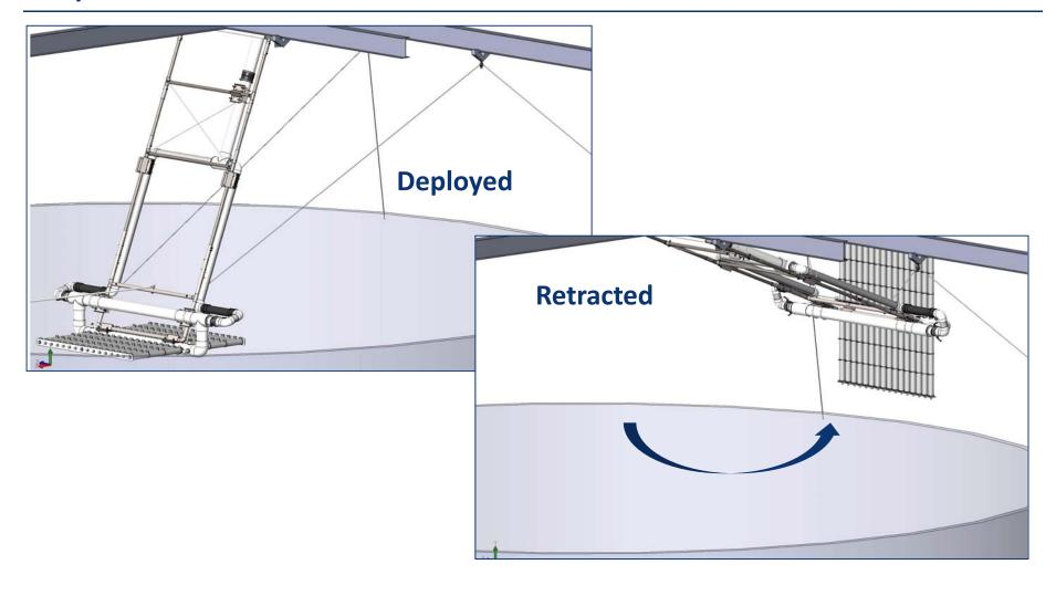
**Device is suspended and retractable**
