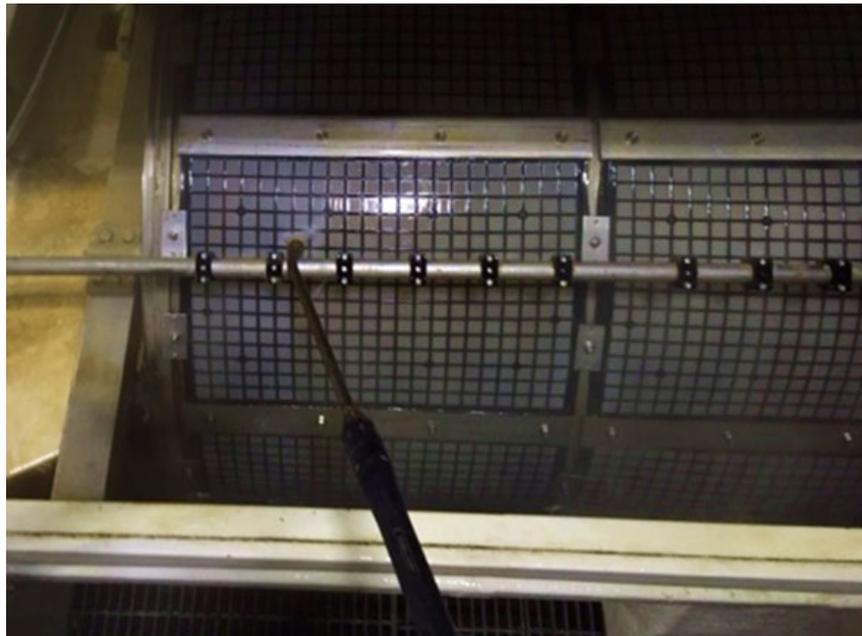
**Figure 7.** Example of a fouled screen being cleaned. Clean screen to the left has already been sprayed and fouled screen remains to the right.
